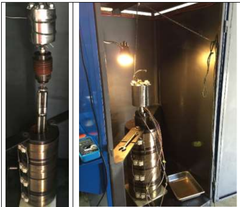
The fixture and plug were placed inside the vessel prefilled with oil. The connections to the controllers were then made.
